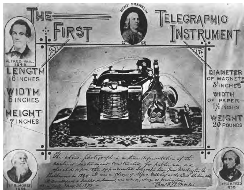
The first telegraphic instrument as created by Samuel F. B. Morse, Alfred Vail, Joseph Henry, and others. THE LIBRARY OF CONGRESS
