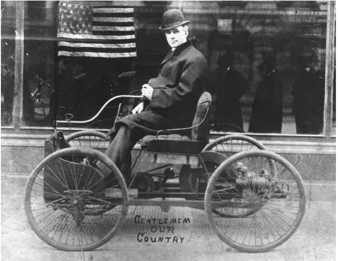
Henry Ford sits in his invention, the Quadricycle. The vehicle had four large bicyclelike wheels, was steered with a system like that in a boat, and had two forward speeds.
